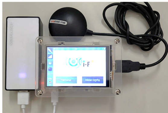
Figure 3. UAI-FI Sniffer: Raspberry Pi 3B, with GPS sensor and Wi-Fi chip
