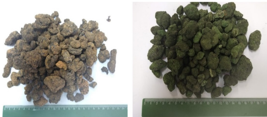
Figure 1. Asphalt rubber pellet samples used in this study - PelletPAVE-Plus (left) and PelletPAV (right)
